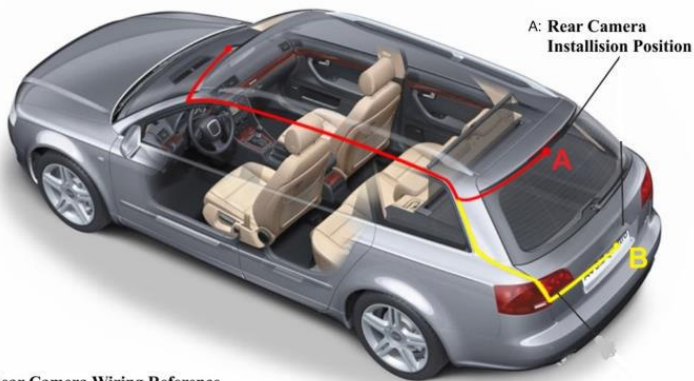
Rear Camera Wiring Reference (as shown above)
